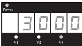
This screen allows the speed of V3 to be adjusted between 600 rpm and 3000 rpm by pressing or holding down either ▲ or ▼ arrow button. Press **DISP/FUNC** button to advance to the next screen.
