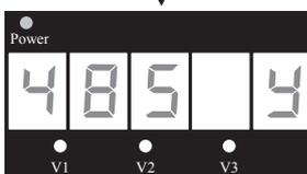
This screen shows that RS485 Control Mode has now been selected. To save this selection, press the **DISP/FUNC** button. The pump will now enter RS485 Control Mode.
