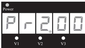
The first Configuration Menu screen is used to adjust the duration of the priming time. Press or hold down either ▲ or ▼ arrow button to adjust the run time between zero and 4 minutes. A setting of zero disables the priming cycle. Press **DISP/FUNC** button to advance to next screen.
