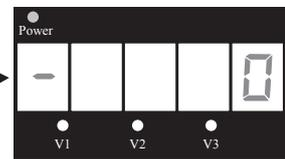
When Prime Mode is active this screen ramps up to 3000 rpm with a rotating circle in block 1
