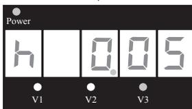
This screen allows the timer of V3 to be adjusted between 5 minutes and 18 hours by pressing or holding down either ▲ or ▼ arrow button. Press **DISP/FUNC** button to advance to the next screen.
