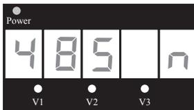
This is the display for RS485 Control Mode selection. The current display shows that RS485 Control Mode is NOT selected and is in "Stand Alone" Mode. To leave the pump in "Stand Alone" Mode press **DISP/FUNC** to exit the Configuration Menu. Press either of the ▲ or ▼ arrow buttons to change modes.
