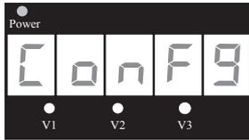
Press and hold the **DISP/FUNC** button for several seconds until the ConFg screen appears.
