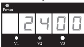
This screen allows the speed of V2 to be adjusted between 600 rpm and 3000 rpm by pressing or holding down either ▲ or ▼ arrow button. Press **DISP/FUNC** button to advance to the next screen.
