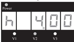
This screen allows the timer of V2 to be adjusted between 5 minutes and 18 hours by pressing or holding down either ▲ or ▼ arrow button. Press **DISP/FUNC** button to advance to the next screen.
