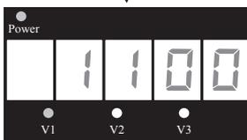
This screen allows the speed of V1 to be adjusted between 600 rpm and 3000 rpm by pressing or holding down either ▲ or ▼ arrow button. Press **DISP/FUNC** button to advance to the next screen.
