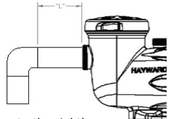
**\*NOTE:** It is recommended that a minimum length of straight piping (shown as "L" in diagram to the right), equivalent to 5 pipe size diameters, be used between the pump suction inlet and any plumbing fittings (elbows, valves, ect).
