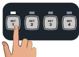
Set point pre-set with unlimited time or configurable with specified time. Editable via panel.
