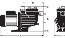
\* Suction and delivery accept 40mm PVC pipe on the I.D. and 50mm fitting on the O.D.
